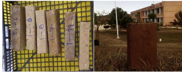
Fig. 3. Appearance and color of the different mixtures prepared for the Echerhirhu-Block.
